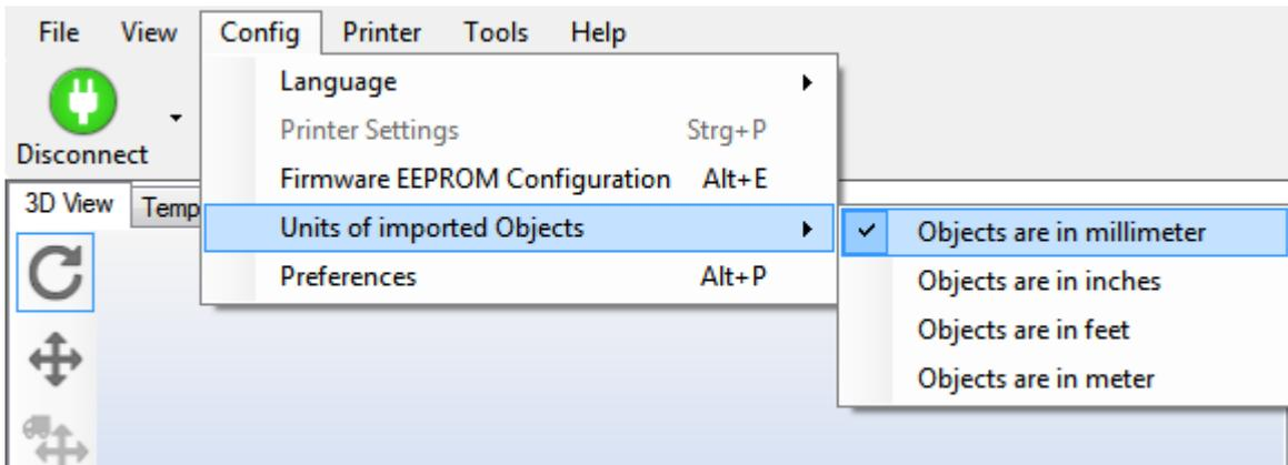
The Repetier-Host uses internally only millimetres. Unfortunately STL and OBJ format do not contain a scaling hint. Therefore you need to select the units used for the creation. That way the Repetier-Host will convert the units correctly into millimetres.
